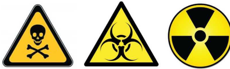
Figure 9 Hazardous Materials Warning Sign
